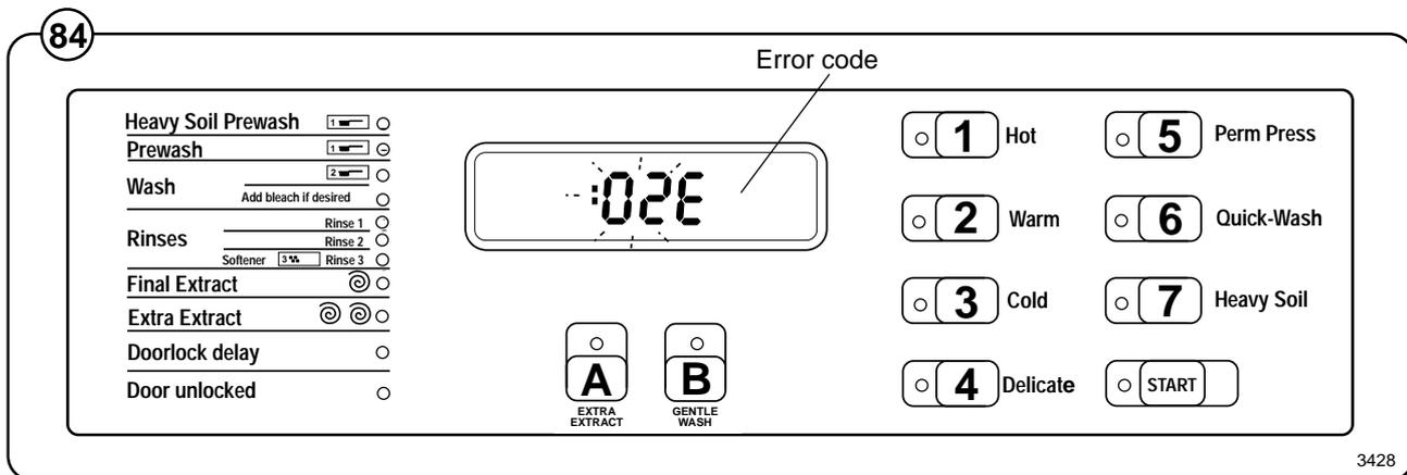
In the case of error codes 01E, 02E, 03E and 14E, an attempt to restart the machine may be made as soon as the fault/error has been remedied, without the power supply being switched off. For the other error codes, a service engineer must be called.
